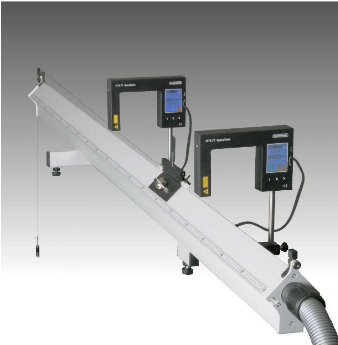
Figure 1: The experimental set-up of Newton's second law of motion.
